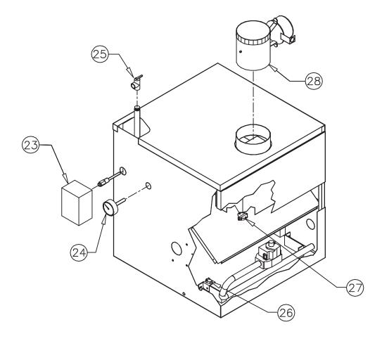
Figure 11.6:Controls/Circulator/Vent Damper
